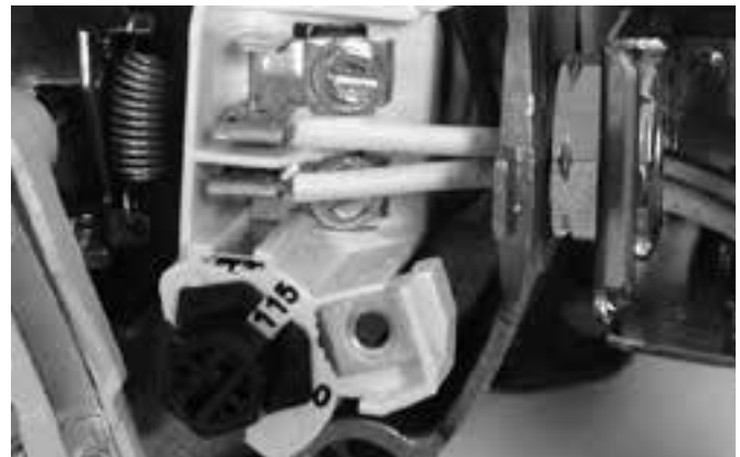
Figure 9: Voltage set to 115 volts, Dial Type
